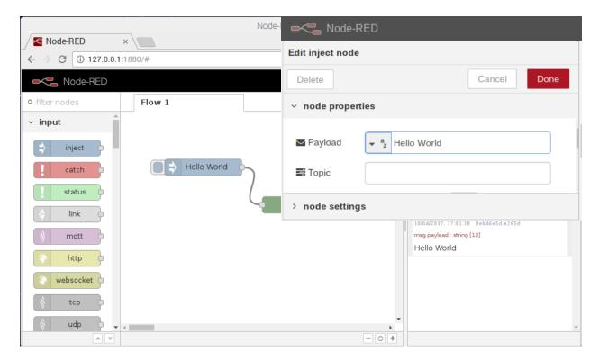
12. Run the flow by clicking on the tab on the left side on the *Hello World* node. Selecting the tab labeled *debug* tab on the right side of the canvas shows the message *Hello World* in the *debug*. Every time the tab on the left side of the *Hello World* node is clicked the message will appear. You have persisted and successfully created a Node-RED program!
